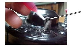
HIGH STRENGTH THREAD LOCKER BEING APPLIED TO LOCK THE NEW STRUT EXTENDERS IN PLACE.
