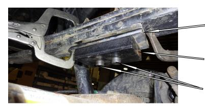
D. INSTALL THE SUPPLIED 1/2" CENTER PIN NUTS AND TOROUE TO 41 FT LBS.
